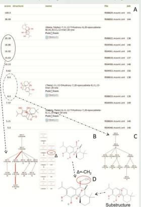
Figure 3: Automatic comparison of spectral trees by the Metitree software A) A list of retrieved hits upon querying the database with an unknown C<sub>21</sub>H<sub>28</sub>O<sub>5</sub> terpenelike compound (Fig. 1B). Two groups of scores around 17.5 and 8.5 are highlighted, of which B) and C) are example spectral trees that belong to rosmanol  $(C_{20}H_{26}O_5)$  (B) and carnosol  $(C_{20}H_{26}O_4)$  (C). D) Based on structural and spectral comparisons, the structure in D is proposed.
