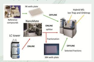
Figure 1: Schematic overview of MS<sup>n</sup> spectral tree data generation.
